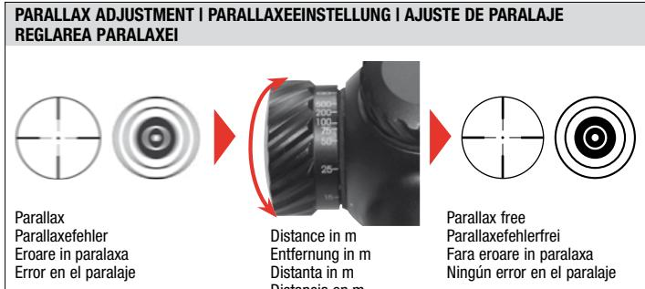
Incorrectly adjusted parallax will cause the reticle to move in front of the target when you look through the scope away from its centre and move the eye behind the ocular. This may cause aiming faults. These can be prevented by correct parallax adjustment which means that the adjustment wheel **10** has to be adjusted according to the appropriate shooting distance. In order to facilitate setting, the ring bears distance markings from 11 yds. (10 m) to  $\infty$  (infinity).
